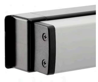
The Axim PR-7200 is a full width, soft touch non-handed panic exit device with a concealed vertical rod which secures the top and bottom of the door. To open the door, the rods are retracted with a turn of a cylinder key or when the touch bar is locked down with an Allen key (dogged).
