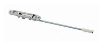
Axim flush bolts secure the slave leaf on double aluminium doors at the top and bottom with a hardened steel 18mm diameter bolt that achieves maximum protection against unauthorised access. To aid assembly, all fixings are included, corners are 2.5mm radiused for easy matching to the cut-out, a centre punch helps locate the centre of the keep and all holes are pre-drilled and countersunk for M fixings.
