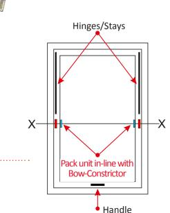
Bow-Constrictor must be fitted centerally at the points X-X to achieve the best seal
