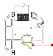
Fit the Sash Spring to the sash on the center line of the stay fixing
