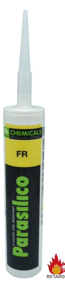
This easy-to-apply fire-retardant, neutral alcoxy curing single-component silicone sealant has been rigorously tested to ensure suitability for use on both horizontal and vertical construction joints in fire secure environments. Parasilico FR silicone foams up in contact with fire and tests prove that it maintains integrity to protect joints for up to 241 minutes in temperatures as high as 1150°C.
