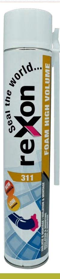
This high-performance polyurethane foam provides a quick and easy way to seal and insulate joints and cracks against heat loss, drafts and noise. ReXon 311 foam will adhere to many common building materials, such as wood, concrete, stone, masonry, plaster, metal, glass, polyester, polystyrene foam and PVC. Please note, this product does not stick to polyethylene film, silicone or PTFE.
