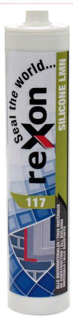
This low modulus neutral oxime curing multi-purpose silicone sticks firmly without primer to most surfaces including PVC, treated wood, aluminium, steel and glass\*, making it ideal for sealing joints in construction and engineering applications. With the use of a primer, reXon 117 can also be used with confidence on alkali surfaces such as concrete and brick.
