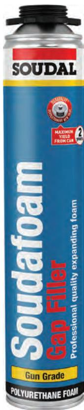
This Soudal gun foam is a one component, self expanding ready to use foam. Suitable for window and door frame installation, filling of cavities and sealing of openings in roof constructions.
