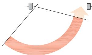
Independent valve screws permit closing speed adjustment from fully open to 15° and 15° to closed.
