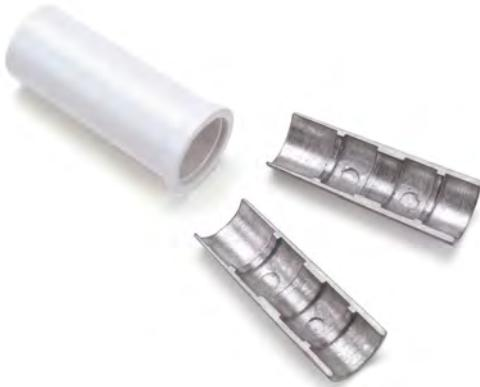
This three-part metal connector is used to connect two lengths of conduit together to create a longer run of conduit. Each connector consists of a two-part metal sleeve and a plastic collar for a secure fit. Available in white, grey and black.
