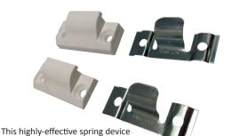
serves two purposes; to improve the seal of a sash on the hinged side of a window and prevent the sash from bowing. Whenever the window is closed, the sash spring pushes against the frame wedge to ensure a firmer seal. Sash-Seal can help to reduce the likelihood of leaking casements on PVCu, timber and aluminium frames, as well as improve their performance and lifespan for reduced call-outs and satisfied customers.
