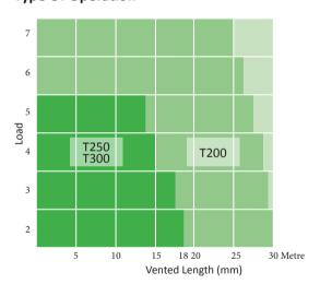
LOAD = No. of chain openers + No. of bends in conduit
