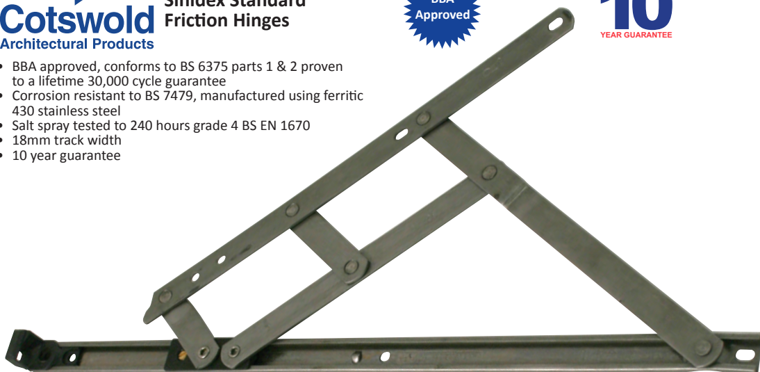
Standard friction hinges 10" shown
