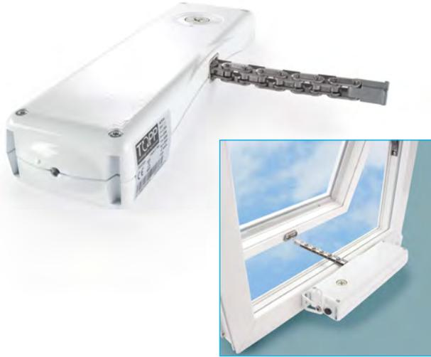
If you want complete control over how far your vents open, then the ACK4 electric chain actuator gives no less than 7 different stroke positions from 100mm up to 400mm, so you can achieve your desired level of ventilation. With a strong die-cast aluminium casing, a robust double-link stainless steel chain and a maximum thrust force of 300N, the ACK4 actuator is a hard-working, reliable choice for your window control system.
