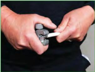
This swage or conduit tool is an essential piece of kit for Highline window control systems. It's used to form the groove in the end of the conduit so it can be securely located into the ridges on the collar of the operator or opener.
