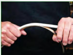
If you're installing Highline manual window controls, you'll need this bend forming tool to create the ideal curve in your conduit with a radius of 90mm for smooth, unhindered cable travel.
