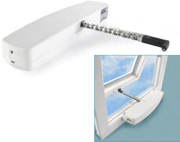
This single-chain actuator comes as standard with a selection of different brackets making it suitable for mounting onto top- and bottom- hung windows. It delivers a maximum push/pull thrust force of 300N which is sufficient to operate most windows, lightweight roof vents and domes. The opening stroke can quickly and easily be adjusted at 200mm or 380mm simply by turning a knob on the outside of the casing.
