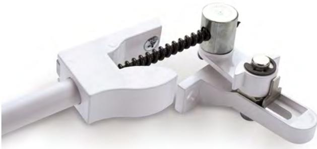
This opener is ideally suited to bottom-hung windows fitted with butt hinges or 'Hopper- style casements that open inwards. It's small enough to fit snugly where space is limited between the reveal and moving frame. Because the moving sash is opened by the strength of the cable alone without the support of any conduit, this opener is better suited to small vents only.
