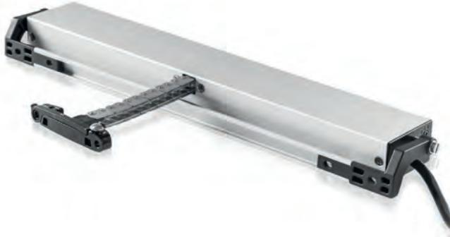
If you need high-level electric window controls for a wide casement, then the Micro EVO actuator is just the job. Its integrated synchronisation function means you can easily link up as many as 4 actuators to work together on single window on site and straight out of the box - no need for a separate sync module.
