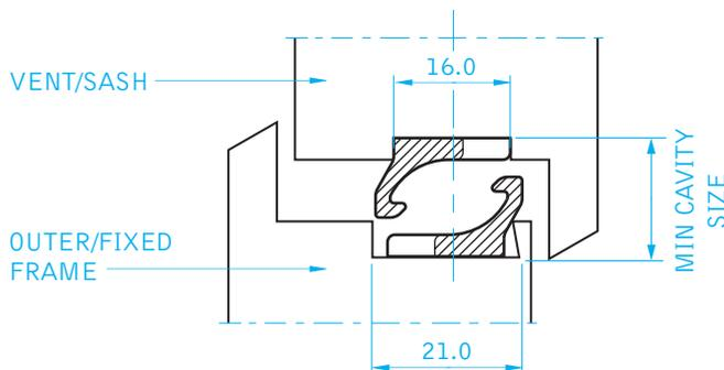
**LOCATE VENT HOOK AGAINST END POINT AND FRAME HOOK AGAINST END CAP**
