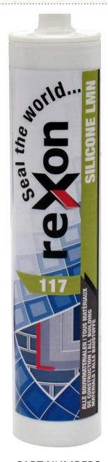
This low modulus neutral oxime curing multi-purpose silicone sticks firmly without primer to most surfaces including PVC, treated wood, aluminium, steel and glass\*, making it ideal for sealing joints in construction and engineering applications. With the use of a primer, reXon 117 can also be used with confidence on alkali surfaces such as concrete and brick.
