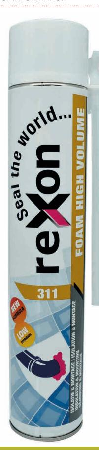
This high-performance polyurethane foam provides a quick and easy way to seal and insulate joints and cracks against heat loss, drafts and noise. ReXon 311 foam will adhere to many common building materials, such as wood, concrete, stone, masonry, plaster, metal, glass, polyester, polystyrene foam and PVC. Please note, this product does not stick to polyethylene film, silicone or PTFE.
