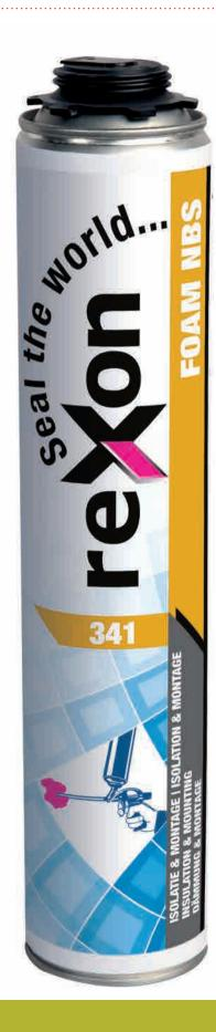
This fast-curing thermal and acoustic insulating polyurethane foam can be used indoors and outdoors to fill holes, cracks and cavities in walls, ceilings and roofs, as well as to insulate pipes, tubes and electrical conduits. It will adhere to most building materials such as wood, concrete, stone, masonry, plaster, metal, glass and many synthetic materials such as polyester, polystyrene and PVC. Please note, reXon 341 will not stick to polyethylene sheets, silicones or PTFE.
