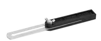
This sliding bevel lets you accurately measure and copy angles. Use the adjustable wing nut to loosen and move the blade until it follows the line of the angle exactly, then tighten the nut to hold the correct angle and transfer it to whatever construction project you're working on.
