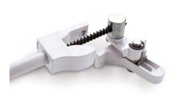
This opener is ideally suited to bottom-hung windows fitted with butt hinges or 'Hopper- style casements that open inwards. It's small enough to fit snugly where space is limited between the reveal and moving frame. Because the moving sash is opened by the strength of the cable alone without the support of any conduit, this opener is better suited to small vents only.
