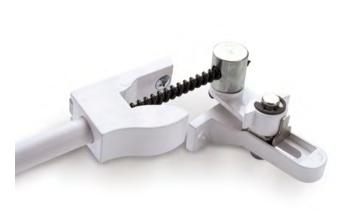
This opener is ideally suited to bottom-hung windows fitted with butt hinges or 'Hopper- style casements that open inwards. It's small enough to fit snugly where space is limited between the reveal and moving frame. Because the moving sash is opened by the strength of the cable alone without the support of any conduit, this opener is better suited to small vents only.
