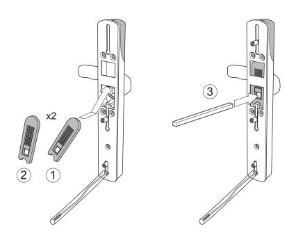
Slide the lug up or down to align with the holes in the door.
