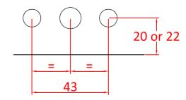
Drill the handle holes to match the appropriate backset.
