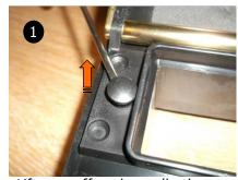
Lift caps off as shown (both ends) It may be helpful to use a small bladed screw driver
