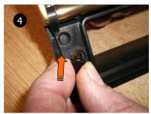
Insert blanking caps from screw pack into boss location hole (both ends)
