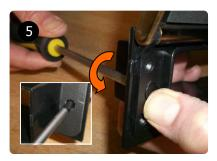
Holding the cap in place, using a cross head screw driver from the back, rotate about 1/8th turn clockwise to secure
