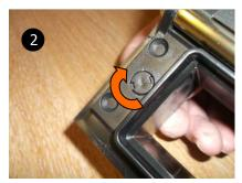
Rotate the boss from the back about 1/8th turn anti clockwise using the fingers to disengage
