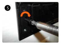
Screw must not be over tightened. Recommended torque setting 3N/m Refer to drill manufacturers data for setting.
