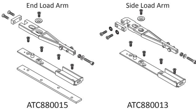
These arms are an essential component of the concealed transom door closer system. Available as either side loading (suitable for use on anti-finger trap doors, armour glass doors and those with a round door stile or narrow door rail) or end loading (for use with anti finger trap doors). These products are fully adjustable, come with hexagonal spanner and feature handy hole and centre lines in channel for easy location of pivot point.
