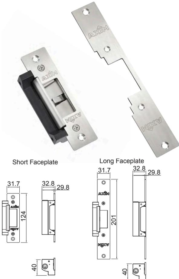
The Axim ES-2200 series of electric strikes are an ANSI style door release designed to work with most leading brand deadlocking night latch locks. They come complete with stainless-steel short and long faceplates for use in most metal or timber door frame applications. The Axim ES-2200 series are shipped as fail-secure and can be converted to fail-safe mode by the simple removal of a screw. The Axim ES-2200 can also be set to 12V or 24V by simply re-configuring the wires in a different sequence.
