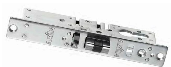
Axim LK-1800 series hook locks and LK-2100 series deadlatches deliver secure locking for a variety of commercial aluminium and steel doors including swing and sliding systems, providing flexible access control during and after business hours. Axim locks and deadlatches are designed to accept euro profile cylinders and are available in three different backsets.
