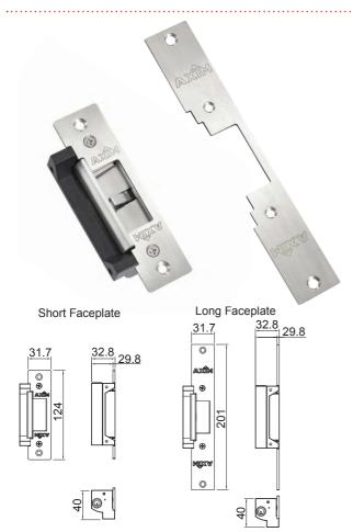
The Axim ES-2200 series of electric strikes are an ANSI style door release designed to work with most leading brand deadlocking night latch locks. They come complete with stainless-steel short and long faceplates for use in most metal or timber door frame applications. The Axim ES-2200 series are shipped as fail-secure and can be converted to fail-safe mode by the simple removal of a screw. The Axim ES-2200 can also be set to 12V or 24V by simply re-configuring the wires in a different sequence.
