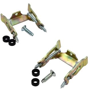
These mounting bridges are recommended for use when fitting the Axim LK-1800 mortice hook lock. They sit inside the master leaf on an aluminium door set and the main lock is screwed to them.
