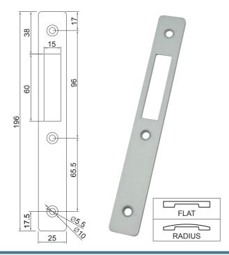
These faceplates are used with Axim's LK-1800 Series Mortice Hook Locks to deliver secure and affordable quality deadlocking on aluminium or steel commercial door installations.
