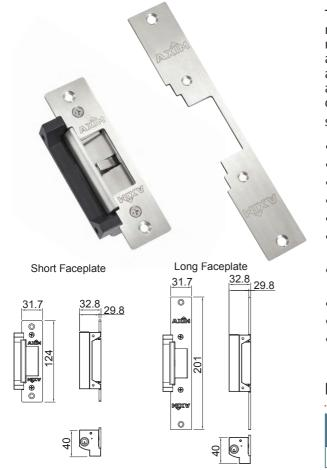
The Axim ES-2200 series of electric strikes are an ANSI style door release designed to work with most leading brand deadlocking night latch locks. They come complete with stainless-steel short and long faceplates for use in most metal or timber door frame applications. The Axim ES-2200 series are shipped as fail-secure and can be converted to fail-safe mode by the simple removal of a screw. The Axim ES-2200 can also be set to 12V or 24V by simply re-configuring the wires in a different sequence.
