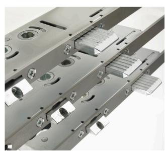
Looking for a super-secure French door lock that's designed to last? The Avantis 550 series multi-point lock offers some of the strongest SBD-accredited and PAS-24 approved reinforcements for double-door sets in the industry. Large opposing chamfered security hooks, a unique triangulated 25mm deep throw centre deadbolt, optional roller cams and strong, laminated high-security shootbolts all add up to even, weathertight compression and ultimate protection against forced entry.
