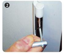
Back the screw off, using a 4mm allen key, by just a small amount (1/3 of a turn approx) to allow up and down movement only. Repeat on all hinges.
