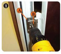
Back off the 2 screws that clamp the slide plate (B) to the frame plate (A)
