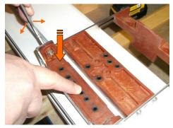
Adjust step height of jig by sliding frame block down until it sits on frame - Tighten with 5mm Allen key
