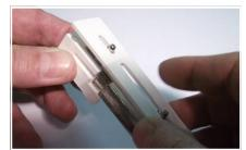
Fit shim as shown if required. Locate the 2 pips into the corresponding holes on the Frame Mount Moulding
