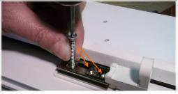
Align location pins with holes in frame, insert the pins and push the Frame Mount fully down. Secure in place with screws in 3 places ensure screws are the correct length to engage with reinforcing
