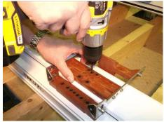
Using a Ø4.0mm drill bit, drill through the skin of the profile only, at the Pin Locations as shown below and as marked on jig
