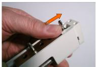
Hinge will normally be supplied unlatched. However, if it is necessary to remove Frame Mount insert flat screwdriver behind metal tang and lever towards Pivot Pin. With screw driver still in place, slide Frame Mount out as shown
