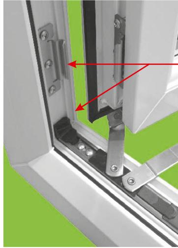
Fit Stay-Guard approx 75mm centres from the internal corner as shown here
