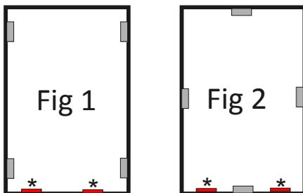
Fit glazing packers on the bottom rail shown marked \*
