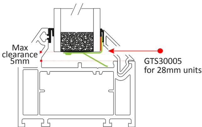
For units up to 900mm width and 1200mm height fit a minimum of 4 GT Snap-Loks see figs 1 and 2
