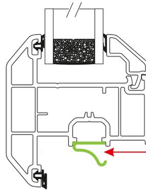
Fit the Sash Spring to the sash on the center line of the stay fixing
