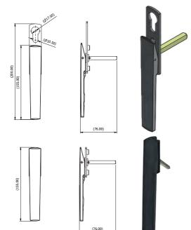
Part of the Glide Hardware folding door hardware range, this sleek and robust bi-fold shootbolt door handle accommodates a cylinder and works with the locking gearbox to operate the shootbolt system and secure the traffic door. Locking handles like these offer excellent crime-beating protection and increased peace of mind to keep security-conscious homeowners and insurance providers happy.
