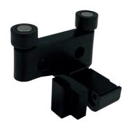
Used when you have an uneven number of bi-fold door panels, the mullion top guide sits in the nylon track at the top corner of a single hinged door panel and works with the mullion roller at the bottom to ensure effortlessly smooth fold and slide operation.
