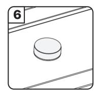
Through fix: from the internal side of the door; screw disc over screw and washer.
