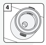
On the pull bar; ensure grub screws are fully out before fitting over boss.
