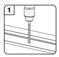
Drill an 8mm hole into the door at the required locations.
