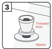
screw followed by the threaded boss (flat base against the door) and tighten with PH3 screwdriver - do not over tighten. Repeat for remaining fixings positions.
