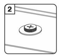
Through fix: from the internal side of the door, slide a clear plastic washer onto the M8 screw and locate onto door, into one of drilled holes.
