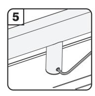
Locate pull bar over the boss, tighten both grub screws on both to secure.
