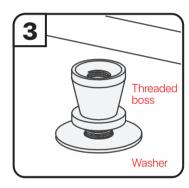
Through fix: From the external side of the door, position a plastic washer over the screw followed by threaded boss (flat base against door)
