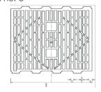
Hollow clay brick HIzW 6-0,7-8DF according to EN771-1 Length/width/height 250 mm/240 mm/240 mm  $f_h \geq 6 \ N/mm^2 / \ \rho \geq 0,8 \ kg/dm$
