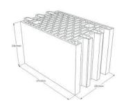
Hollow clay brick Porotherm 25P+W KL15 according to EN771-1 Length/width/height 373 mm/250 mm/238 mm  $f_{D} \geq$  12 N/mm² /  $\rho \geq$  0,9 kg/dm³
